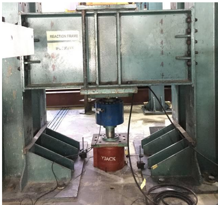
Figure 1(c) Pile Connector mounted on the UTM Machine prior to Compression Test
