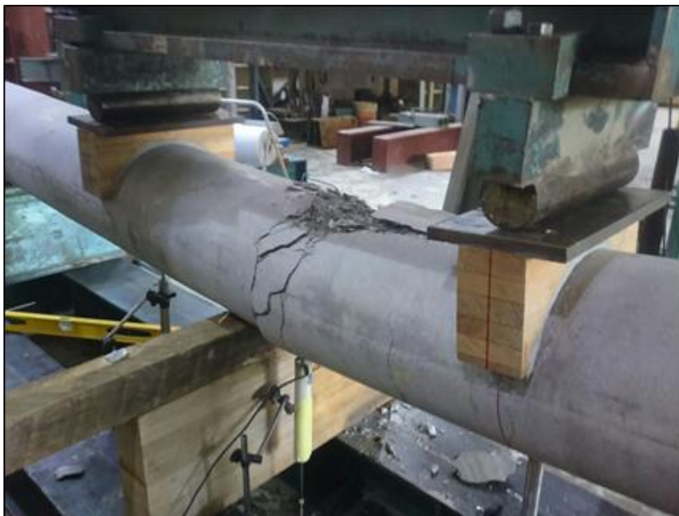
Figure 3(b) Failure Test Mod under Bending Test for SC300 Ø (pile body)
