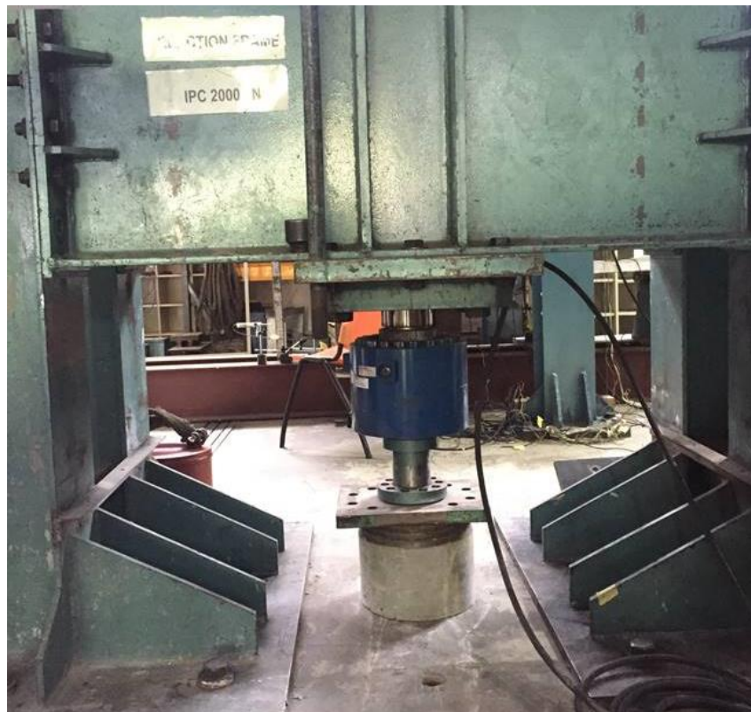
Figure 1(b) Pile Body mounted on the UTM Machine prior to Compression Test
