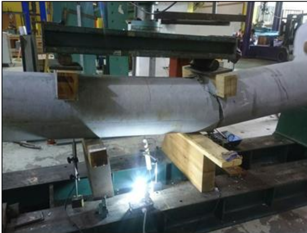
Figure 5(b) Failure Test Mod under Bending Test for SC400 Ø (pile body)
