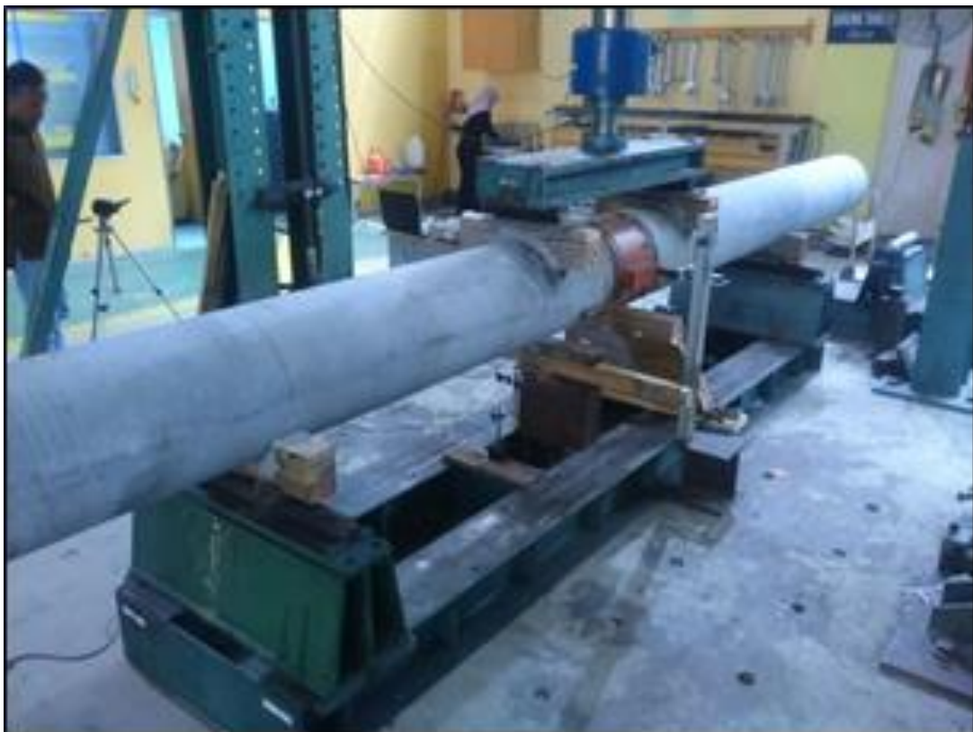
Figure 2(c) YJACK Connected to Pile mounted on the Roller Supports prior to Bending Test.
