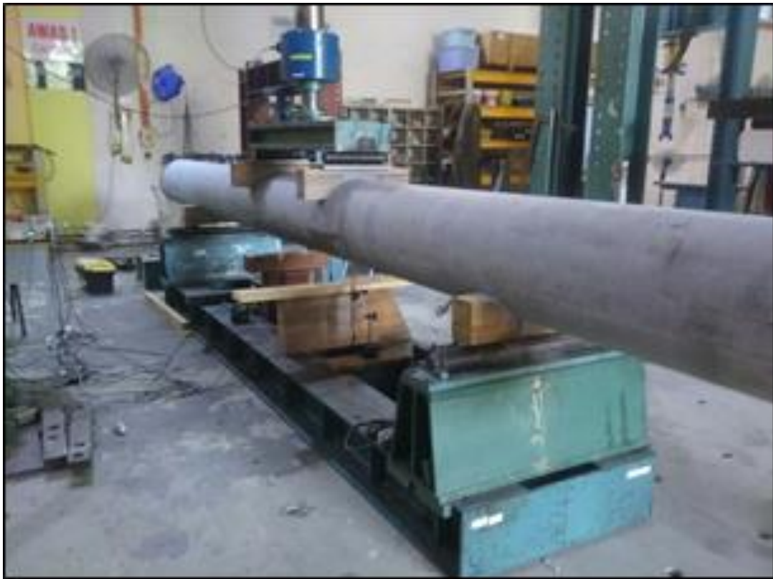
Figure 2(b) Pile Body mounted on the Roller Supports prior to Bending Test.
