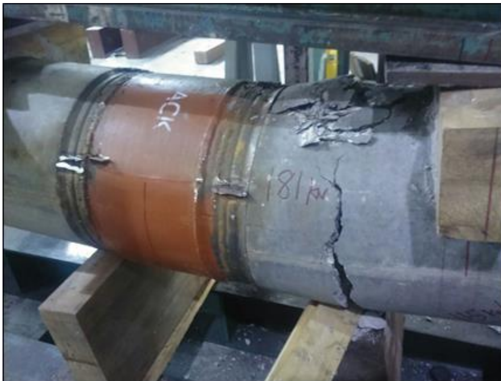
Figure 6(b) Failure Test Mod under Bending Test for YJ400 Ø (YJACK Connector), failure occurred at concrete
